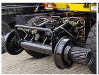
As option available: Friction Drive System available for 1404 ZW with track width 1000 and 1435 mm.
